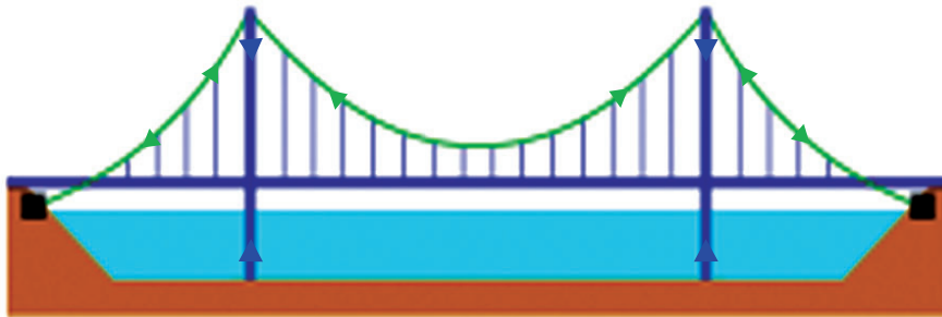
Figure 14: Forces acting on a suspension bridge
